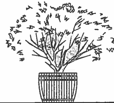
Wooden Barrel Planter: Wooden Barrel Saw Cut to a Height of 2'-0". Base Dimension of 2'-0" Diameter.
